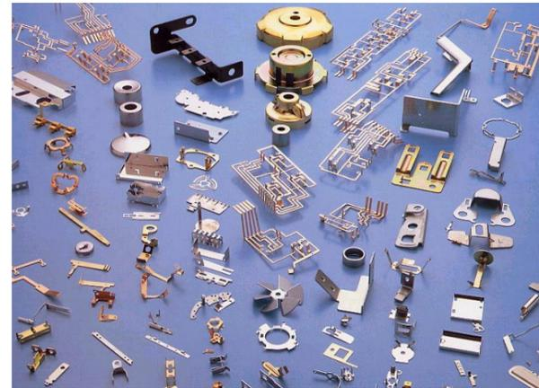
被加工材 SPCC,SAPH,SECC,SPG,LSS,SUS304,SUS430,SUS631
