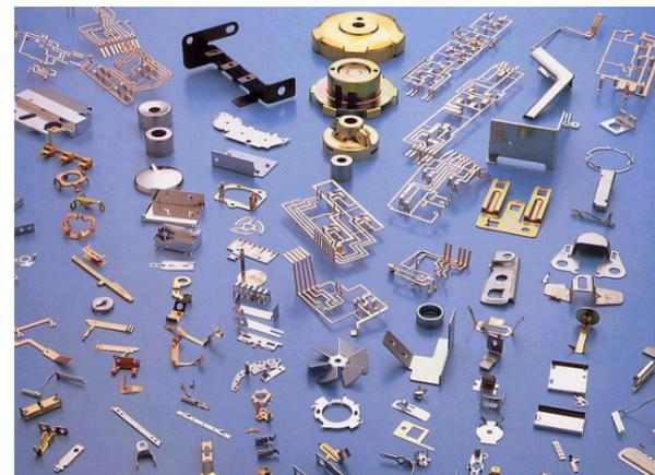
被加工材 SPCC,SAPH,SECC,SPG,LSS,SUS304,SUS430,SUS631
